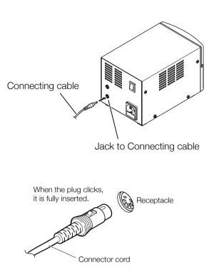
Push the plug in as far as it will go, and try to remove it without pressing the release pin. If it stays in the receptacle, it is properly seated.
